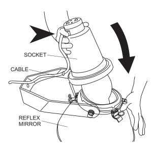
Figure 11. Positioning the Socket
